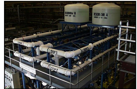
Distribution System Simulator - Top View
