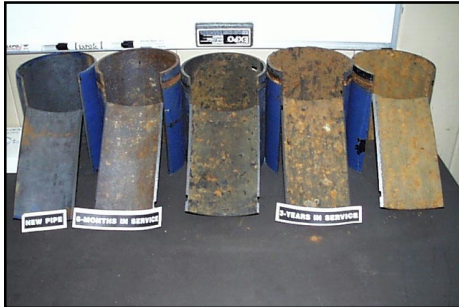
Pipe deterioration over time
