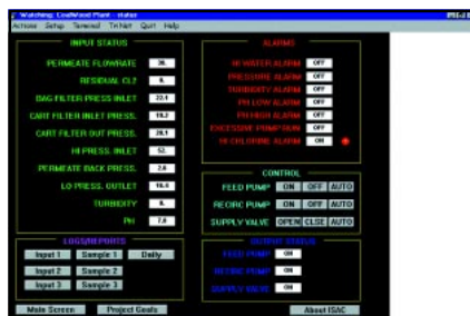
Remote Monitoring/Control Interface.
