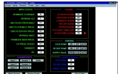
Remote Monitoring/Control Interface.
